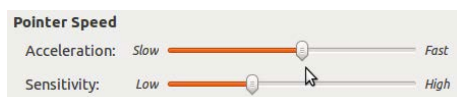
Figure 10: Ubuntu 10.10 configuration interface. A help page says about the first slider: “Use the slider to specify the speed at which your mouse pointer moves on your screen when you move your mouse”. About the second: “Use the slider to specify how sensitive your mouse pointer is to movements of your mouse”.
