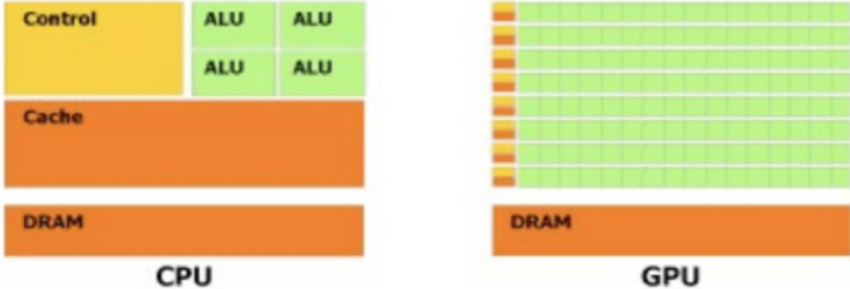
Figure 1-2. The GPU Devotes More Transistors to Data Processing
