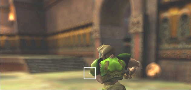
Figure 2: Quake III video game with Depth-of-Field blur effect implemented. The white square corresponds to the auto-focus zone that follows the user's focus point measured by eye-tracking.
